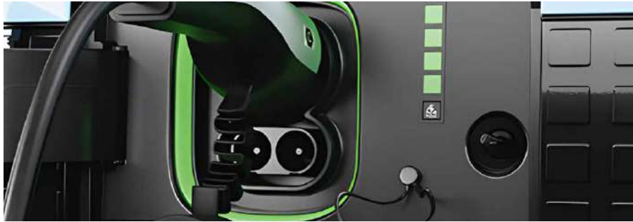
Charging port with multi-colour surround light and state-of-charge (SOC) indicator
